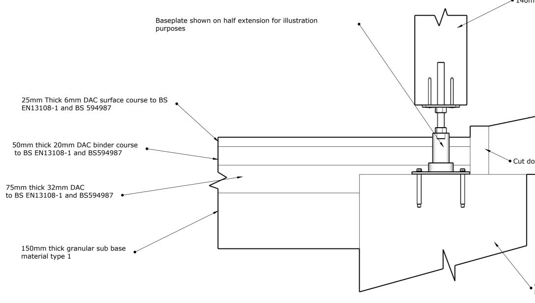
Note: Could we arrange for our building to be 20mm smaller on both depth and width to overcome the issues? As you can see from the detail, the post is 140mm and the baseplate is 160mm, the edgings are being installed to the frame size, hence the 10mm clash with the edgings.
