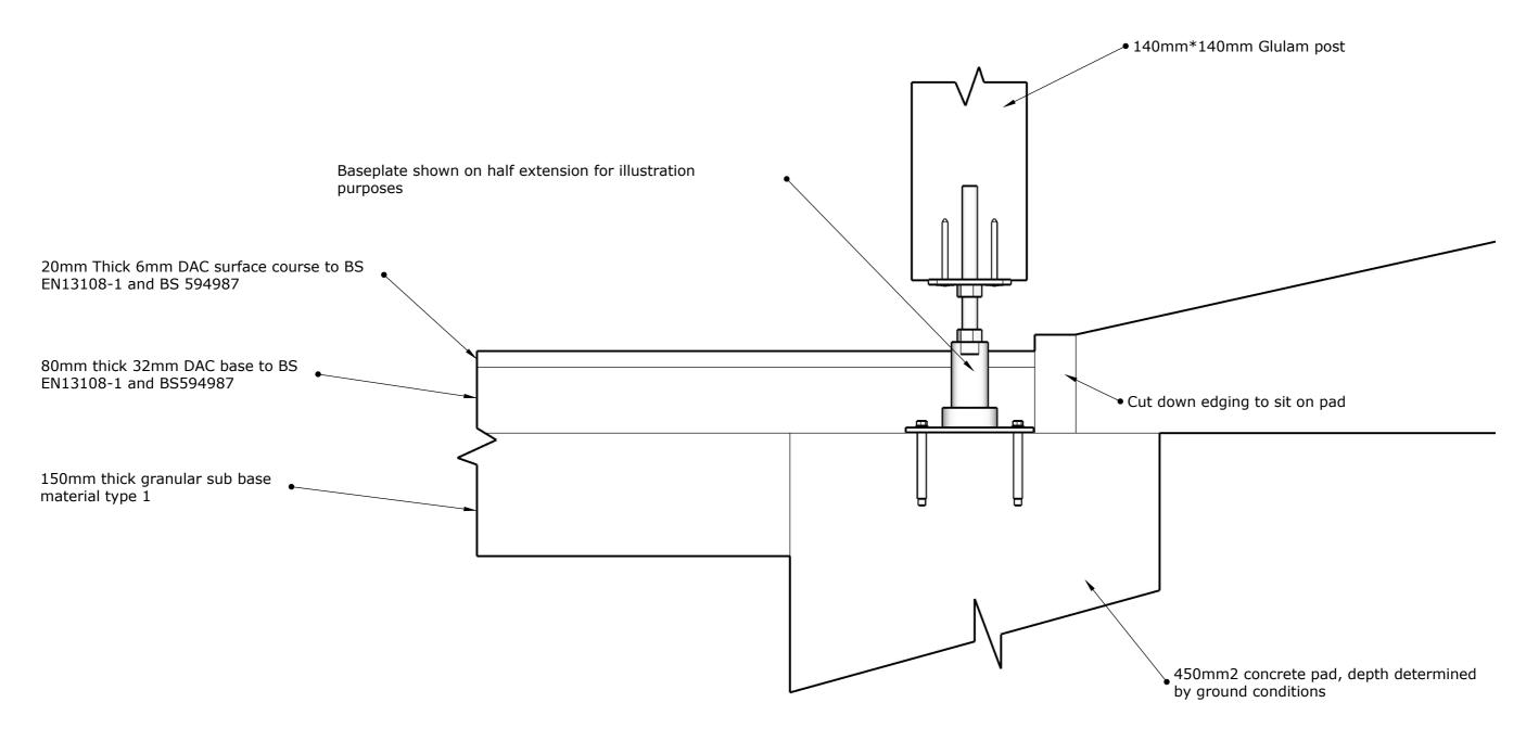
Note: Could we arrange for our building to be 20mm smaller on both depth and width to overcome the issues? As you can see from the detail, the post is 140mm and the baseplate is 160mm, the edgings are being installed to the frame size, hence the 10mm clash with the edgings.
